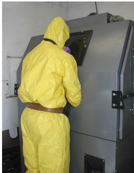
Figure 6. Isolated cabinet for NORM decontamination.
